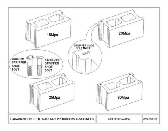
Most assuredly, the structural designer is not ignorant to the requirements for CMU marking in material standard CSA A165.1. A cross-reference is contained in a note to Clause 15.1.2 of CSA S304.1-04, "Design of Masonry Structures". CSA S304.1-04 is used by the structural engineer for the structural design of masonry:
