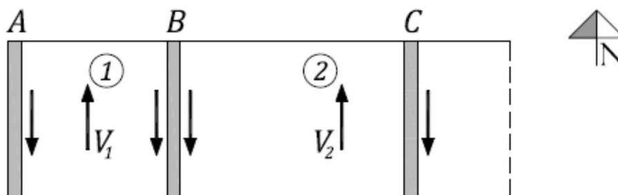
Figure 1-13. Plan view for analysis of flexible diaphragm.
