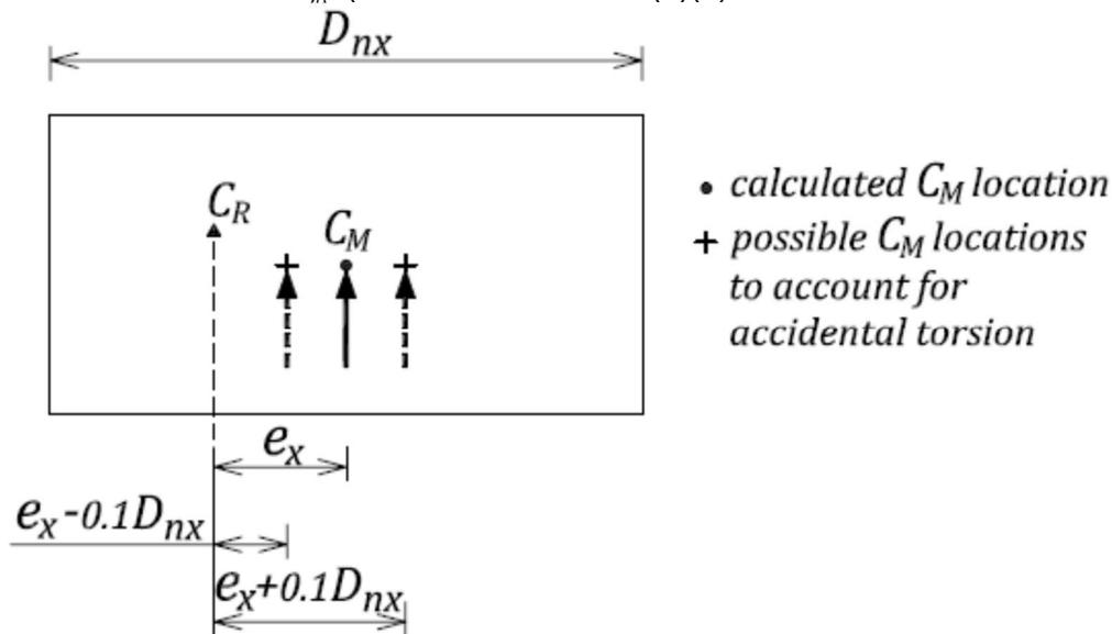
Figure 1-10. Torsional eccentricity according to NBC 2015.
