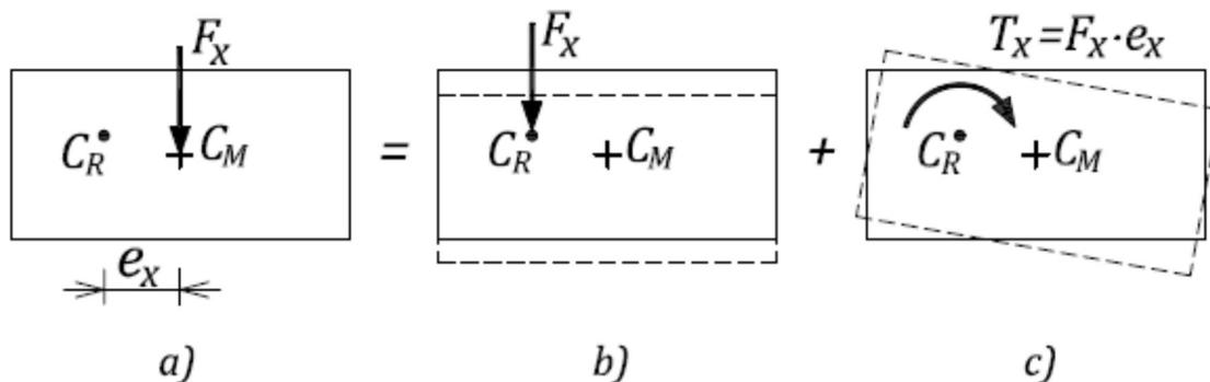
*Figure 1-8. Torsional effects a), can be modelled as a combination of a seismic force,  $F_x$ , at point  $C_R$  (causing translational displacements only) b), and a torsional moment,  $T_x = F_x \cdot e_x$  (causing rotation of building plan) about point  $C_R$  c).*
