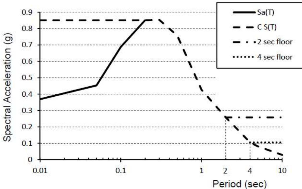
Figure 1-2. Log plot of the UHS  $S_a(T)$  and the Design Spectrum  $S(T)$  spectrum for Vancouver with limits in the short and long period regions.
