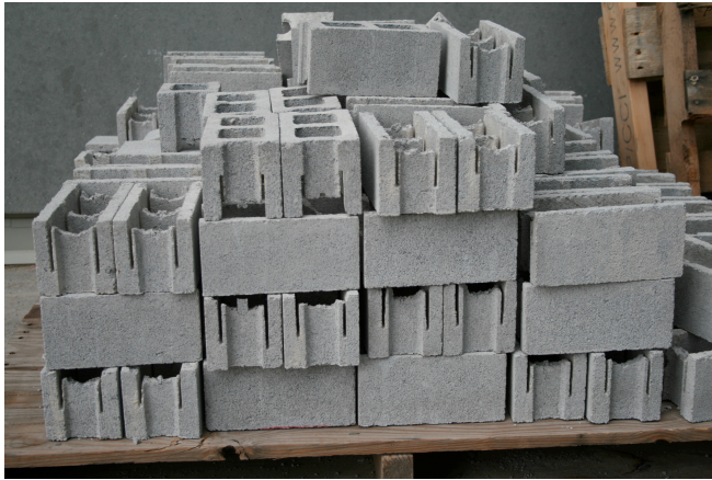
Half size blocks cut to resemble knock-out blocks
