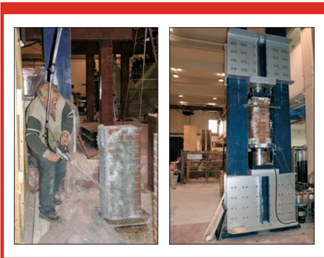
Glass fibre-reinforced polymer (GFRP)-wrapped brick column testing is being performed at the University of Calgary.
