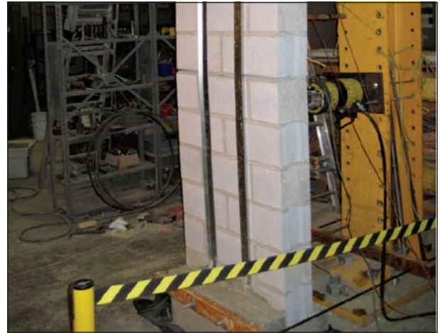
This external steel stud reinforced hollow block foundation wall is being tested at McMaster University in Hamilton.
