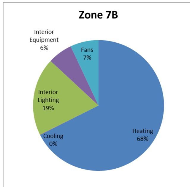
**Figure 20 Annual Energy Use of the Canadian Baseline Warehouse (NECB-11 Prescriptive Configuration- No FDWR Adjustments) Zone 7B.**
