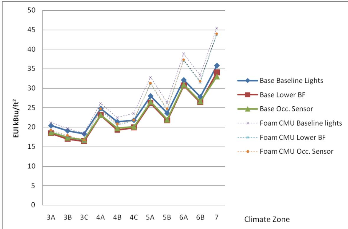
**Figure 15. Effects of Lighting System Alternatives on Yearly Energy Use.**
