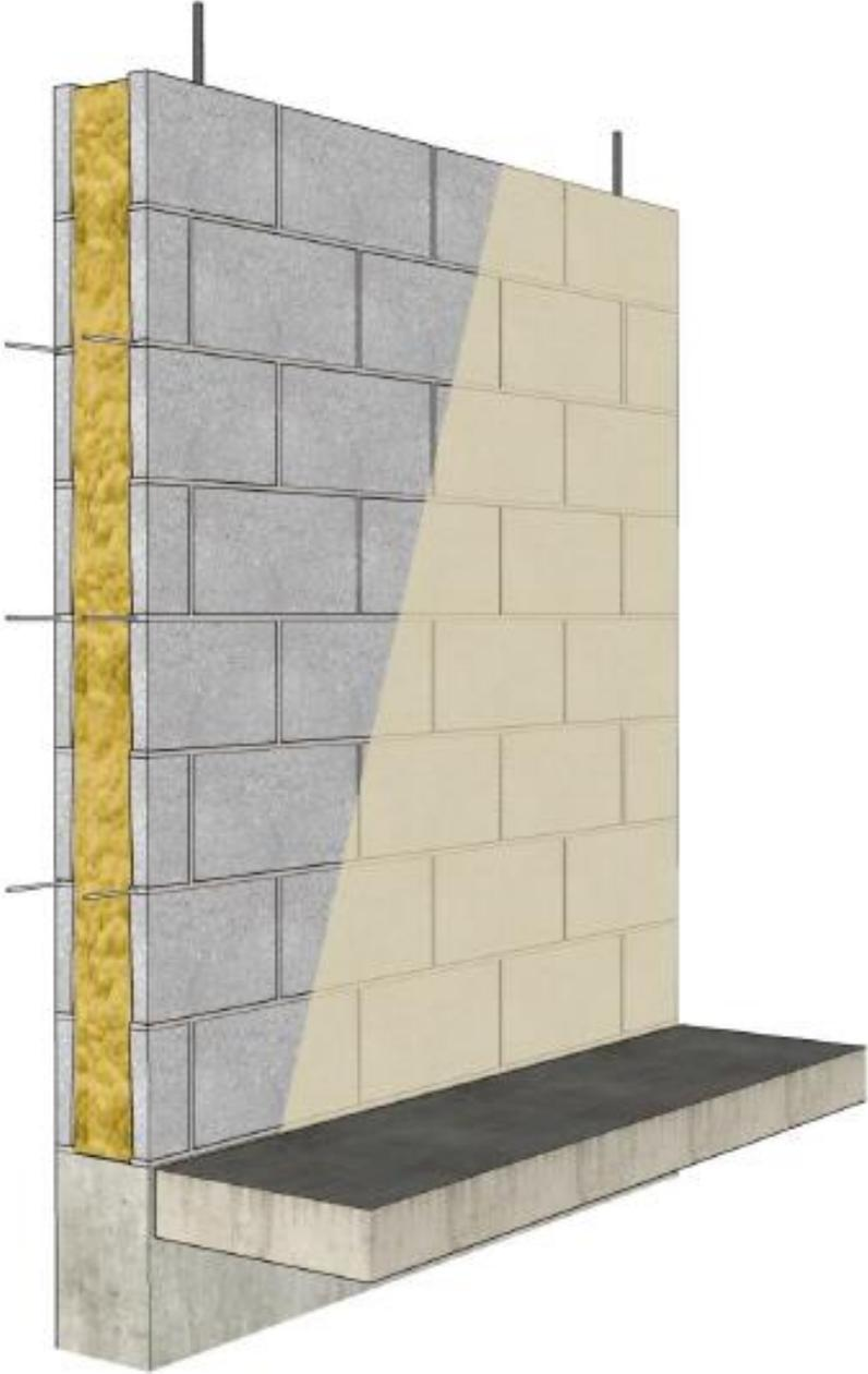
**Figure 14. Exterior Masonry Wall Sections with Core Insulation.**
