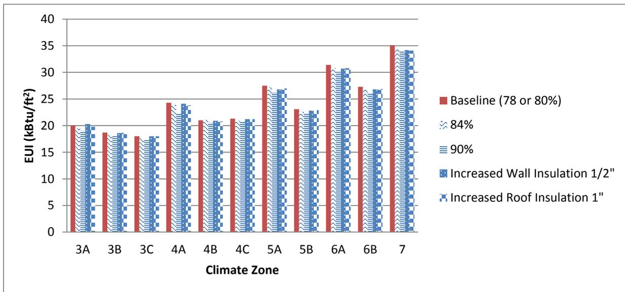
**Figure 13. Energy Use Intensities: Wall and Roof Insulation vs. Heating Efficiency.**
