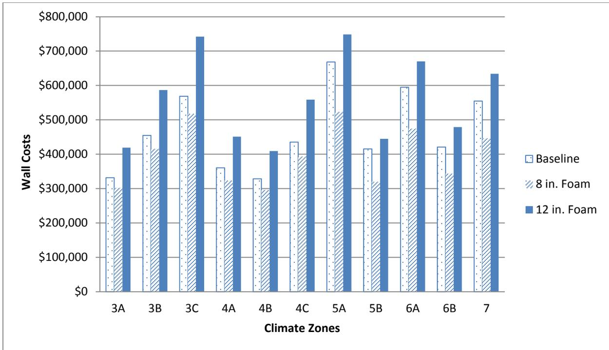
**Figure 17. Wall Configuration Costs for the Warehouse Building.**
