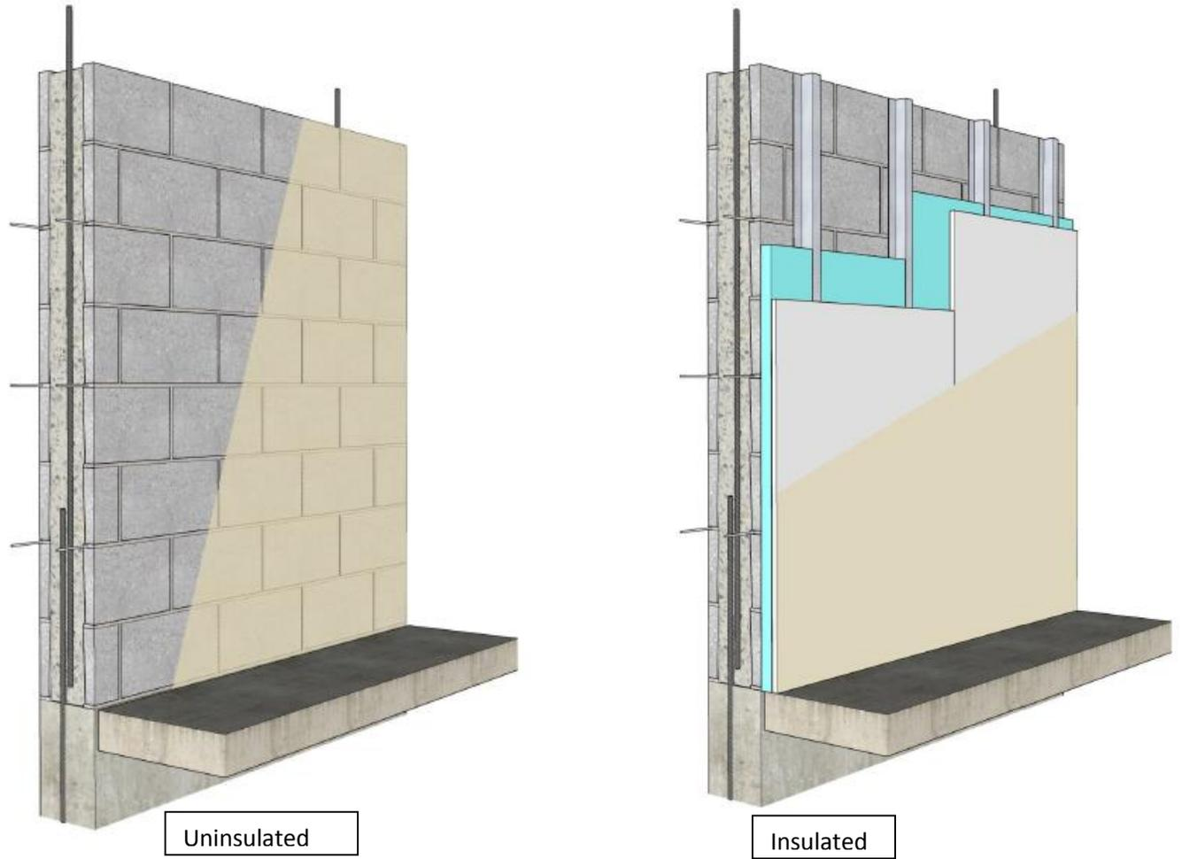
**Figure 11. Exterior Masonry Wall Sections, Uninsulated and Insulated.**
