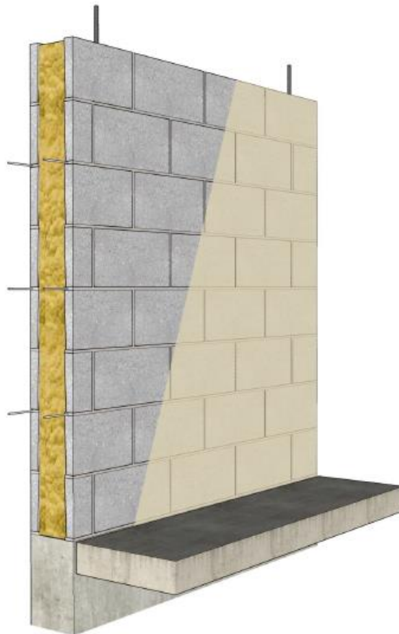
Figure 17. Exterior Masonry Wall Sections With Core Insulation.
